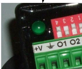
+V is the positive terminal for power supply.
