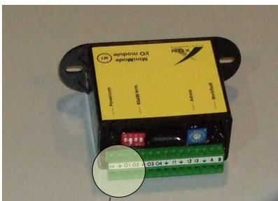
The device must be powered with a DC voltage in the range 10-30 volts. The current consumption is 150 mA for the device itself, plus the consumption of the attached loads, up to 4 amperes.
